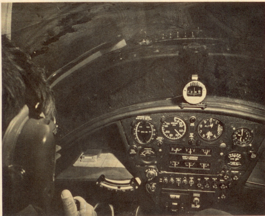
J-2's cockpit in flight. About only controls different from those in fixed-wing craft are rotor-engagement handle on firewall aft pilot's head and helicopter-like lever at far left of left seat.
